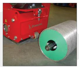
A full drum of eighty blades is shown removed from the new BMC-335EHY-R. The number of blades used can be adjusted with spacers to achieve the desired shaving width or pattern.
